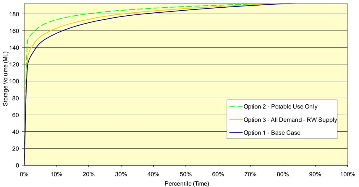
**Figure 5 Hobble Gully Dam – Water Storage Percentile Analysis**
