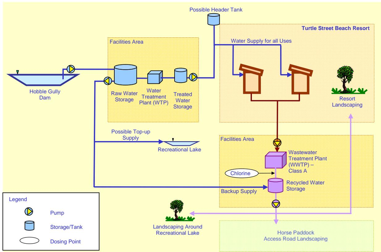
**Figure 7 Water Management Schematic**
