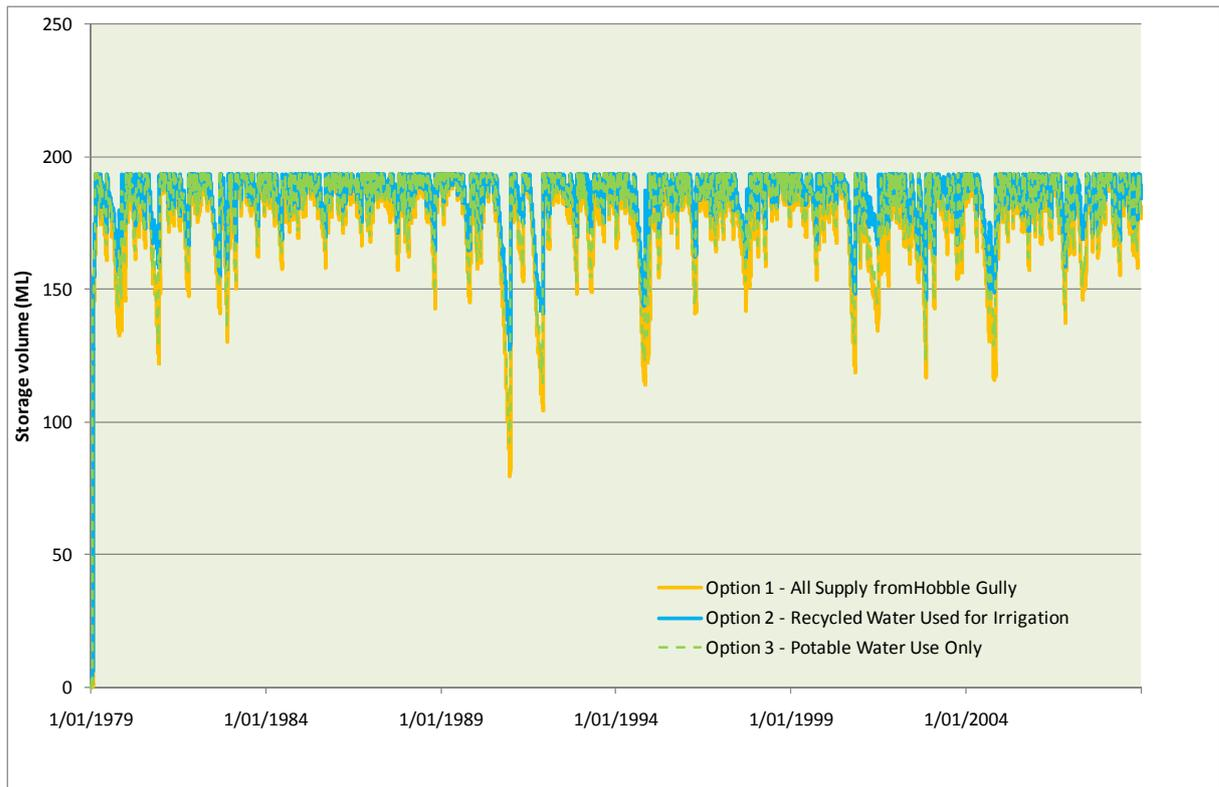
**Figure 4 Hobble Gully Dam – Water Storage Variation Over Time**
