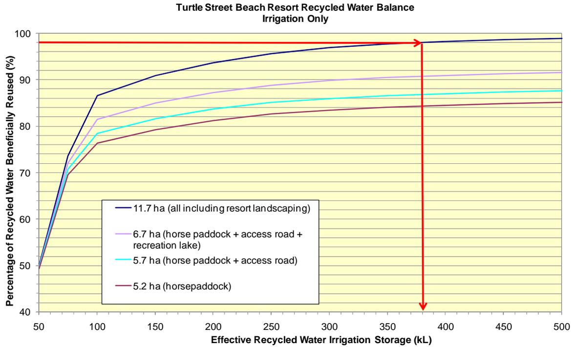
**Figure 6 Recycled Water Balance Model Results**
