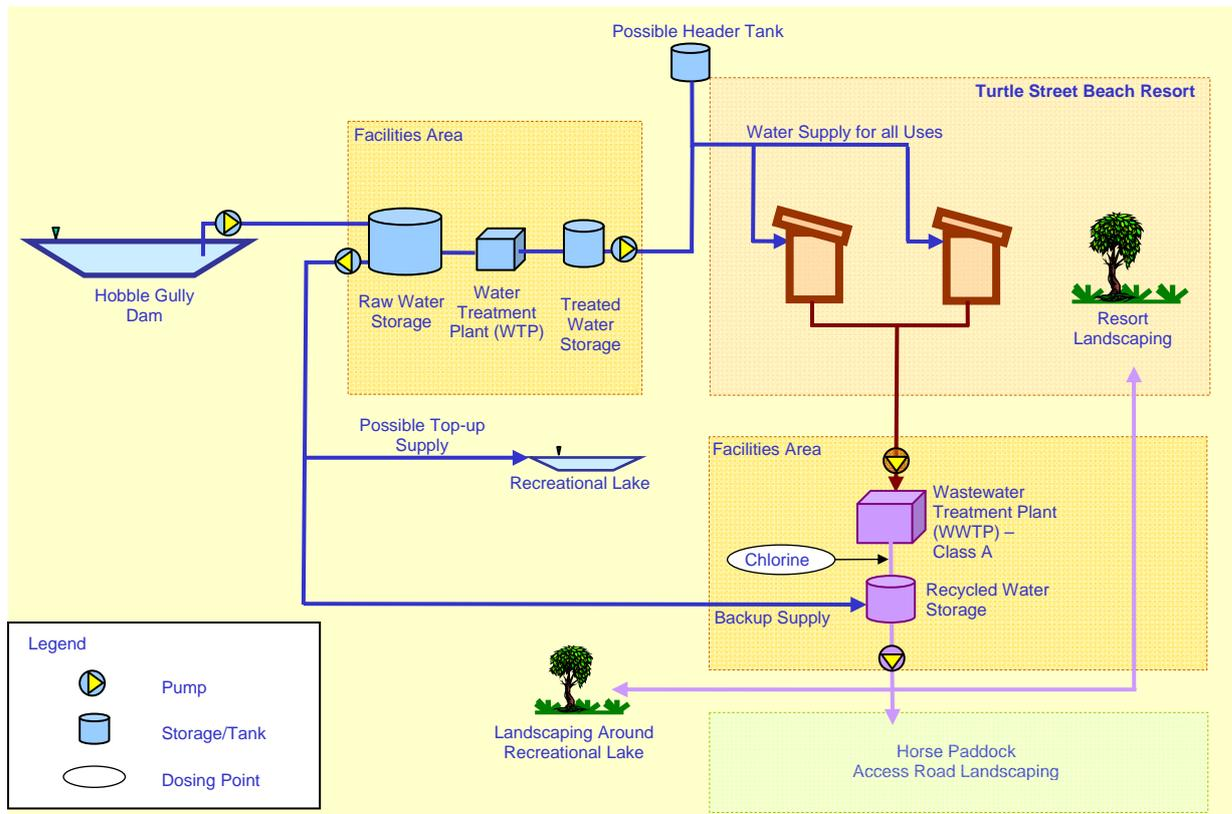
**Figure 7 Water Management Schematic**
